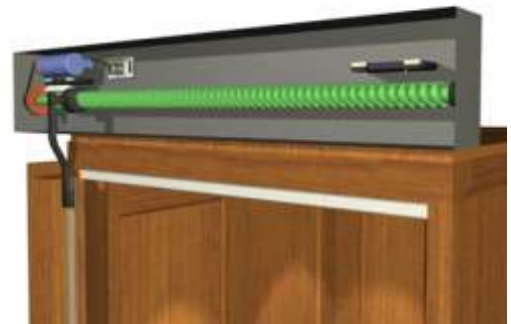
Operator in Open Position
